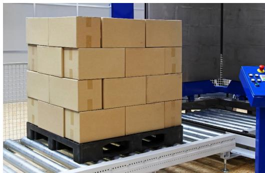
Pallet Conveyor allows efficient transport, accumulation, lifting and sorting of heavy loads as an alternative to forklifts handling. In warehouse automation operations a pallet conveyor is generally utilized to move loads of several hundreds kilograms while ensuring continuous feed of work and cutting edge efficiency. The high-performance synchronous brushless servomotor, coupled with planetary gearbox, ensures performance with loads up to 1500 kg per zone.
