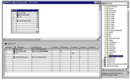
Use the mouse to select the desired hardware components from the **Catalog** and drag them into the station window.
