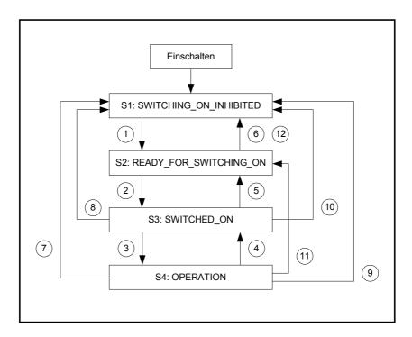
Figure 9.9: Simplified state diagram
