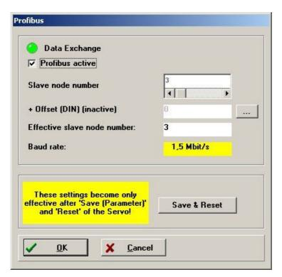
Figure 8.8: Setting of operating parameters
