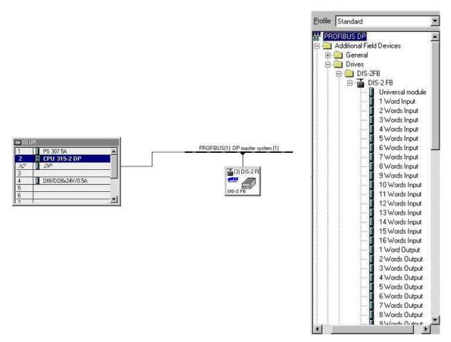
Figure 5.3: Hardware configuration under SIEMENS S7
