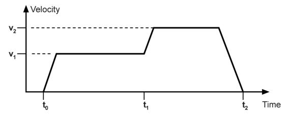
Figure 11.11: Uninterrupted sequence of motion tasks
