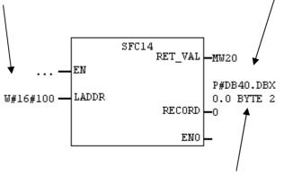
Initial address within the DB (0.0) and number of bytes received (20 bytes)
