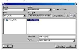
Select the project name in the **Name** field of the **Open** window. Then select **SIMATIC 300(1)** in the right window pane. Then click on the **OK** button to open the hardware configuration of your project.
