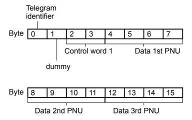
Figure 5.2: Example of the telegram format for the DUET\_FL 48/10 FB
