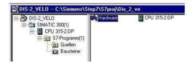
The command **Options->Install new GSD...** adds the GSD file MME0A38.gsd, which is required for adding the DUET\_FL 48/10 FB to the hardware catalog.
