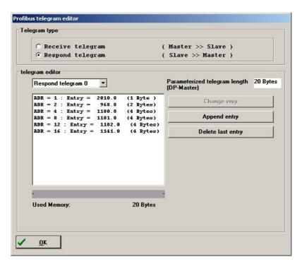
Figure 6.5: Composition of a response telegram
