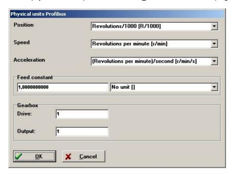
Figure 7.6: Setting of physical units
