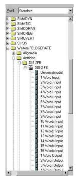
The telegram length has to be taken into consideration when selecting the modules. This means:
