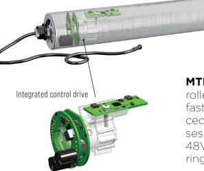
MTR 46 AD is today the most powerful motorized driven roller on the market, delivering 75W power ratings, enabling faster movement and higher payload capacity. Its advanced gearless direct drive design minimizes mechanical losses, reduces energy costs, and ensures quiet operation. The 48Vdc power supply enhances efficiency and simplifies wiring.
