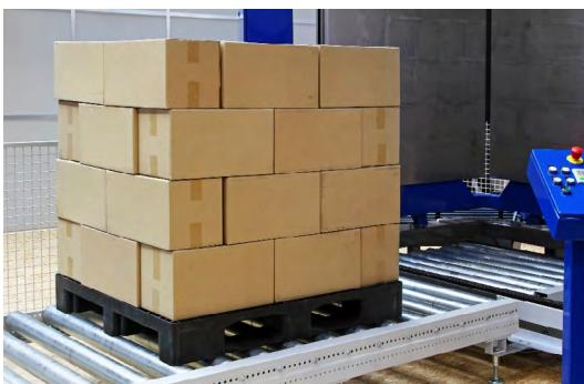
Pallet Conveyor allows efficient transport, accumulation, lifting and sorting of heavy loads as an alternative to forklifts handling.
