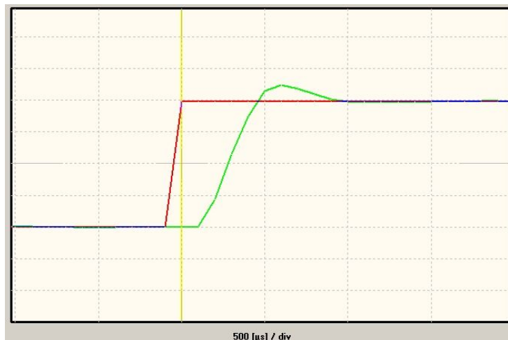
Figure 1: Current controller step response
