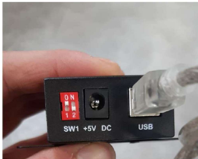
Figure 8: USB adapter dip switch
