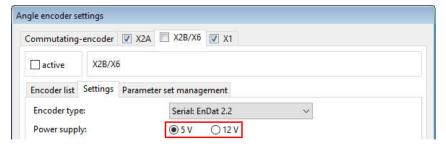
Figure 25: Angle encoder settings: Parameterisation of supply voltage
