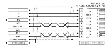
Figure 18: Pin assignment: motor connector (motor temperature sensor) [X6]
