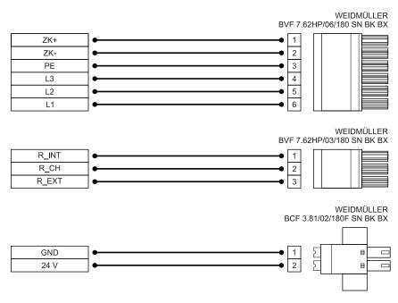
Figure 15: Pin assignment: "power supply connector [X9], [X9A], [X9B]"
