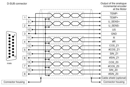
Figure 26: Pin assignment: analogue incremental encoders [X2B]
