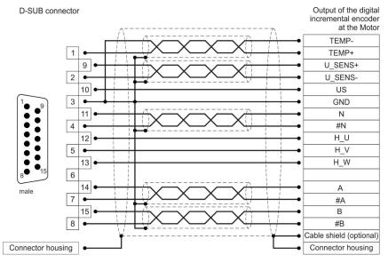
Figure 28: Pin assignment: digital incremental encoder (RS422) [X2B]
