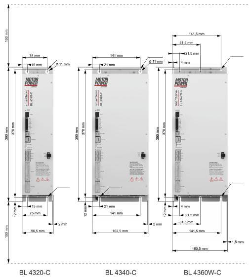
Figure 9: Dimensions and installation clearance BL 4320-C...BL 4360W-C
