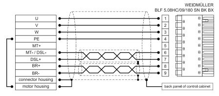
Figure 19: Pin assignment: motor connector (HIPERFACE DSL®) [X6]
