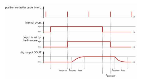
Figure 35: Filter time mechanism in the case of digital outputs
