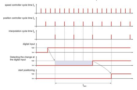
Figure 34: Filter time mechanism in the case of digital inputs
