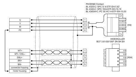
Figure 22: Pin assignment: motor connector (motor temperature sensor) [X6], [X6A]
