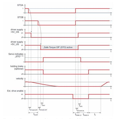
Figure 37: Time response of the activation of the STO safety function with a restart
