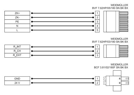
Figure 13: Pin assignment: "power supply connector [X9]"
