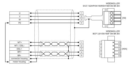
Figure 20: Pin assignment: motor connector (motor temperature sensor) [X6], [X6A]
