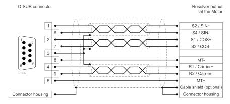
Figure 24: Pin assignment: resolver connector [X2A]
