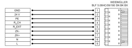
Figure 11: Pin assignment: "power supply connector [X9]"
