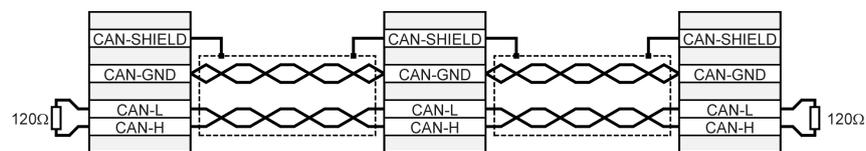
Figure 32: CAN bus cabling example
