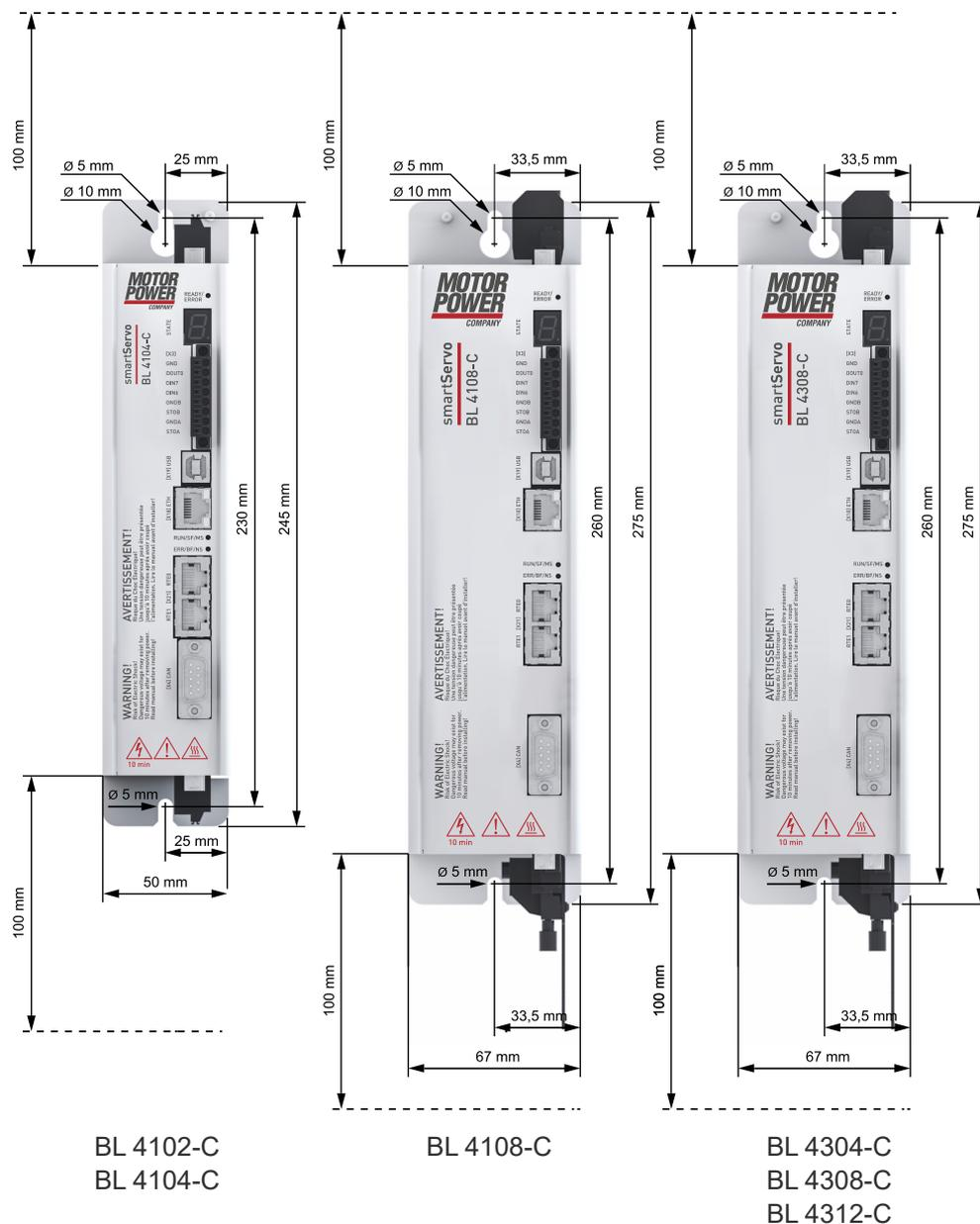
Figure 8: Dimensions and installation clearance BL 4102-C...BL 4312-C
