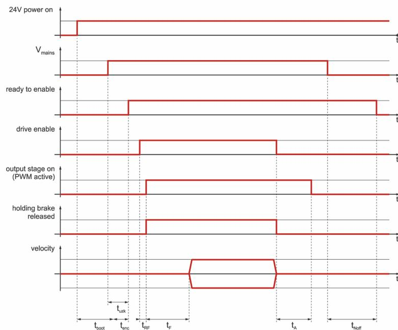
Figure 36: Time diagram of the servo drive
