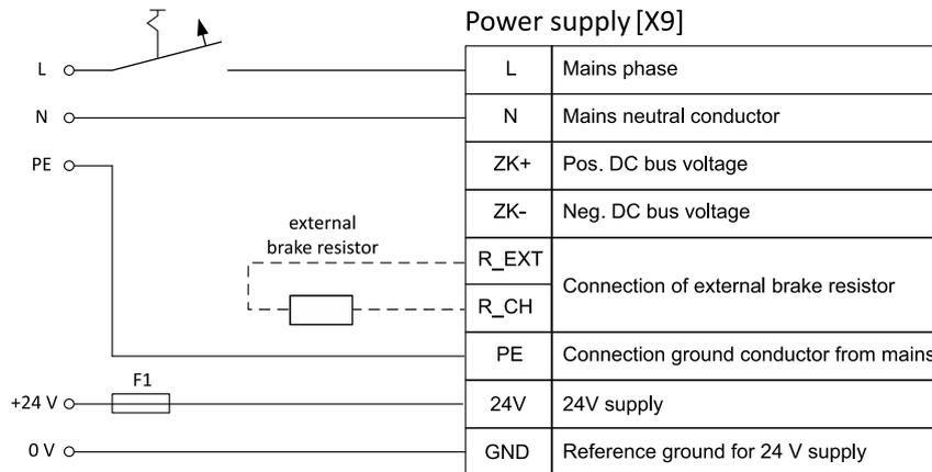
Figure 10: Connection of a BL 4102-C/BL 4104-C to the power supply [X9]
