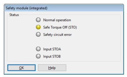
Figure 128: "Safety module (integrated)" window
