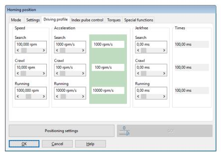
Figure 46: "Homing position" window - "Driving profile" tab
