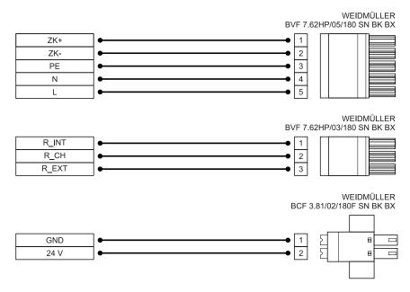
Figure 136: Pin assignment: "power supply connector [X9]"
