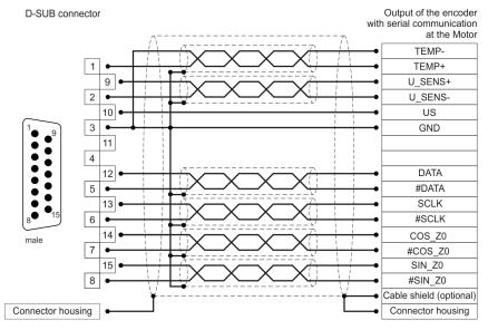
Figure 150: Pin assignment: incremental encoder with a serial interface [X2B]
