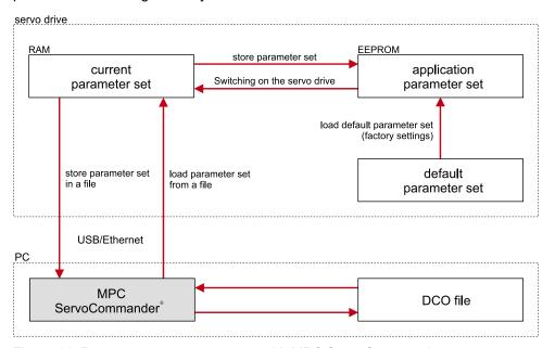
Figure 80: Parameter set management with MPC ServoCommander
