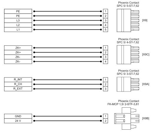
Figure 140: Pin assignment: "power supply connector [X9], [X9A], [X9B], [X9C]"
