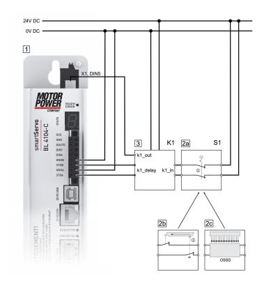
Figure 125: Circuit example "Deceleration and safe torque switch-off" (SS1, "Safe Stop 1") (single-phase servo drive)
