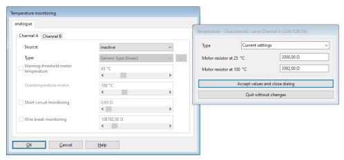
Figure 120: Temperature characteristic - linear sensor
