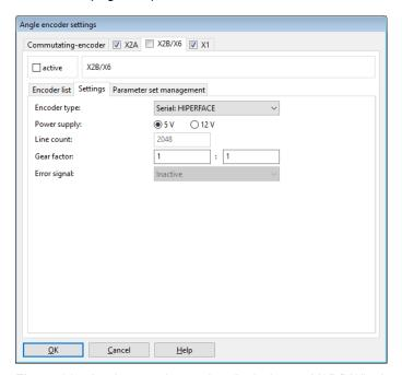
Figure 90: "Angle encoder settings" window – "X2B/X6" tab - "Settings - Encoder type: Serial: HIPERFACE"
