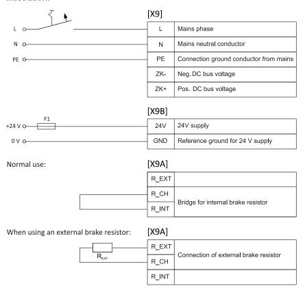
Figure 135: Connection of a BL 4108-C to the power supply [X9]
