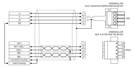
Figure 144: Pin assignment: motor connector (HIPERFACE DSL®) [X6], [X6A]
