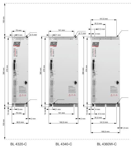
Figure 132: Dimensions and installation clearance BL 4320-C...BL 4360W-C
