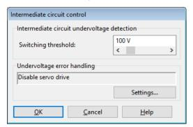
Figure 115: "Intermediate circuit control" window
