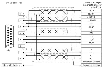
Figure 151: Pin assignment: digital incremental encoder (RS422) [X2B]
