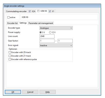
Figure 88: "Angle encoder settings"" window - "X2B/X6" tab - "Settings" - "Encoder type: Analogue"
