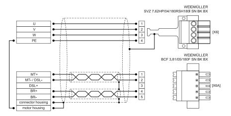
Figure 143: Pin assignment: motor connector (motor temperature sensor) [X6], [X6A]
