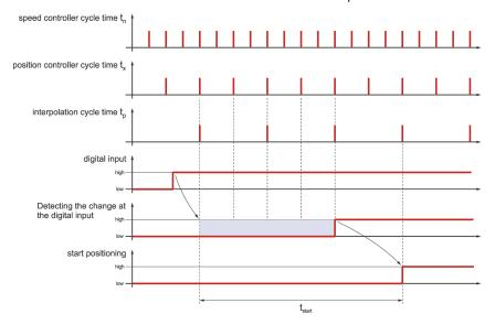
Figure 157: Filter time mechanism in the case of digital inputs
