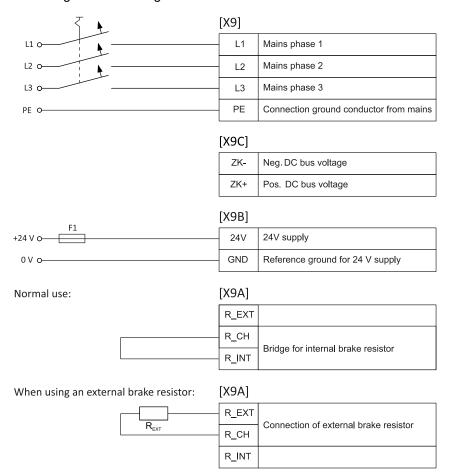
Figure 139: Connection of a BL 4320-C, BL 4340-C or BL 4360W-C to the power supply [X9]
