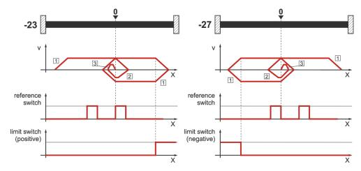
Figure 42: Reference switch with an initial movement in the positive and negative direction
