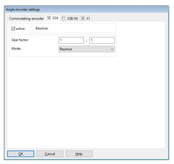
Figure 84: "Angle encoder settings" window - "X2A" tab
