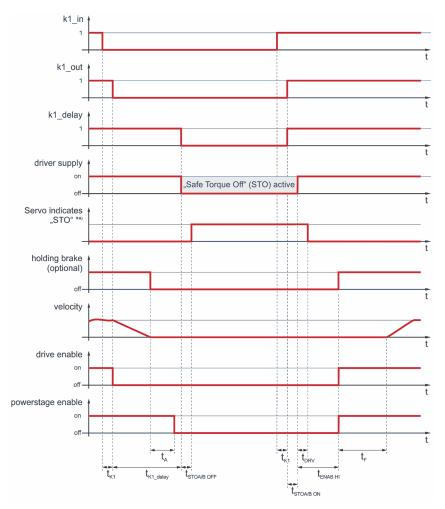
Figure 161: Time response during the activation of the SS1 safety function (external switching) with a restart
