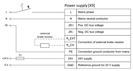
Figure 133: Connection of a BL 4102-C/BL 4104-C to the power supply [X9]
