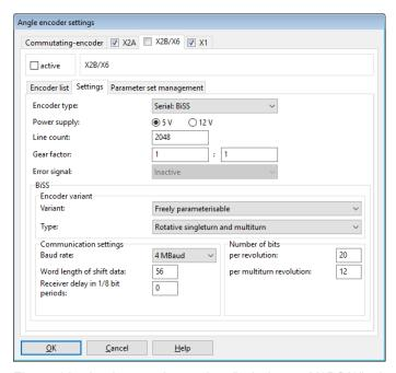
Figure 92: "Angle encoder settings" window – "X2B/X6" tab – "Settings" – "Encoder type: Serial: BiSS"
