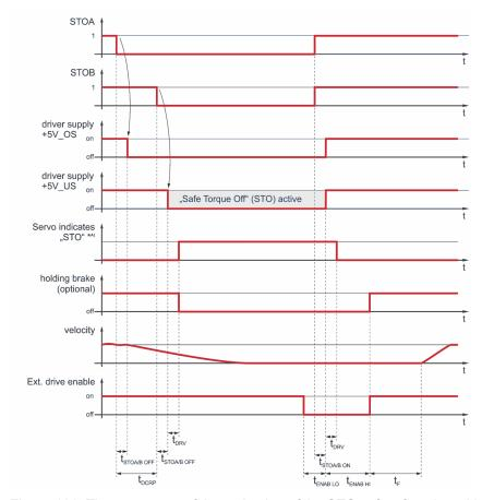
Figure 160: Time response of the activation of the STO safety function with a restart
