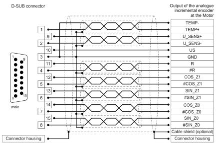
Figure 149: Pin assignment: analogue incremental encoders [X2B]
