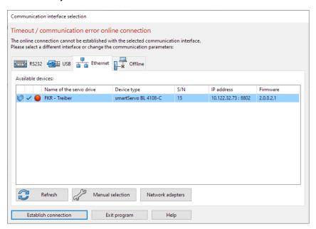
If a communication connection can be established, this is signalled by a check mark ( ) next to the device status. A communication connection can then be established by double-clicking on the desired servo drive or clicking on the Establish connection button. If this check mark is not displayed, the servo drive cannot be reached. This is the case, for example, if it is located in a different subnet.
