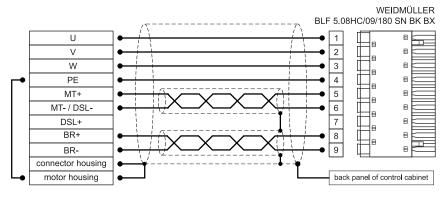
Figure 141: Pin assignment: motor connector (motor temperature sensor) [X6]
