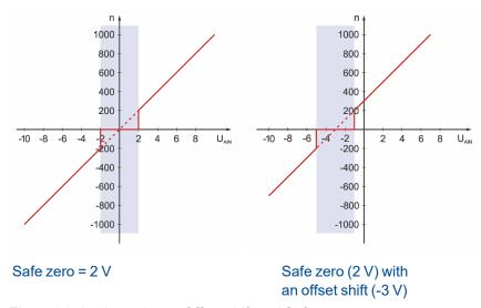
Figure 34: Analogue input: Offset shift and Safe zero
