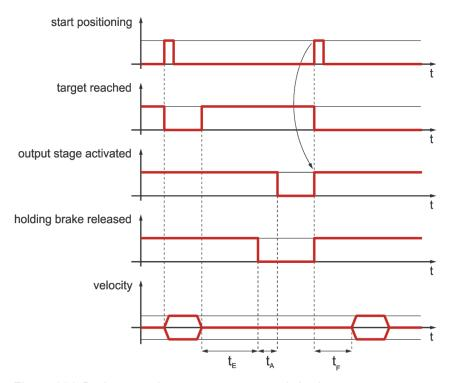
Figure 114: Brake control parameters: automatic brake
