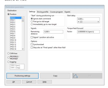
Figure 71: "Destination parameters" window - "Settings" tab
