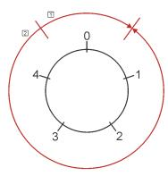
Figure 73: Rotary motion in the rotary axis mode
