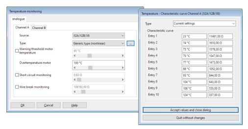
Figure 121: Temperature characteristic - non-linear sensor
