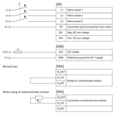
Figure 137: Connection of a BL 4304-C, BL 4308-C or BL 4312-C to the power supply [X9]
