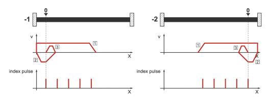
Figure 37: Homing run to the stop with index pulse evaluation
