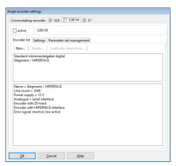
Figure 85: "Angle encoder settings" window - "X2B/X6" tab - "Encoder list"
