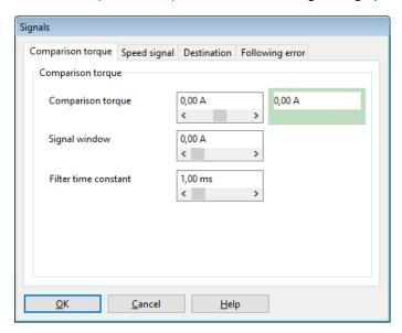
Figure 103: "Signals" window - "Comparison torque" tab
