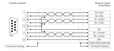
Figure 147: Pin assignment: resolver connector [X2A]
