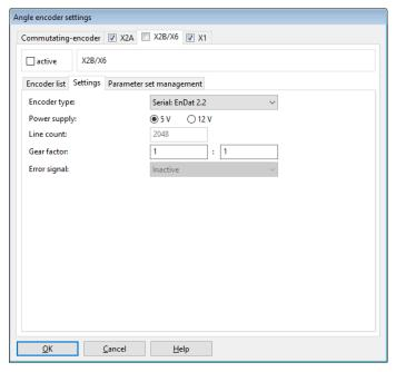
Figure 89: "Angle encoder settings" window – "X2B/X6" tab - "Encoder type: Serial: EnDat 2.2"
