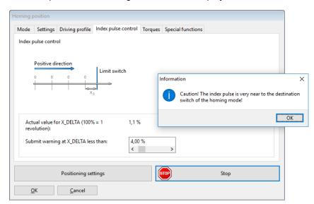
Figure 47: "Homing position" window - "Index pulse control" tab
