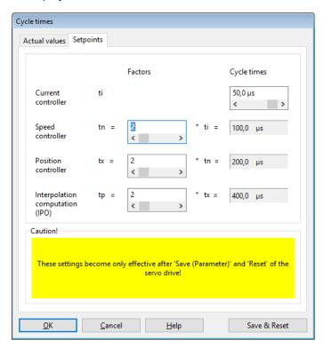
Figure 116: "Cycle times" window - "Setpoints" tab
