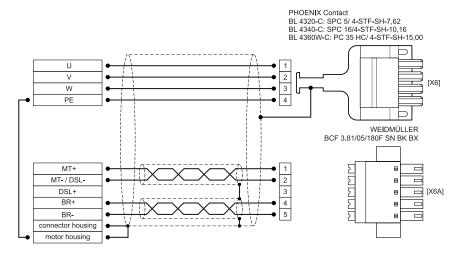
Figure 145: Pin assignment: motor connector (motor temperature sensor) [X6], [X6A]
