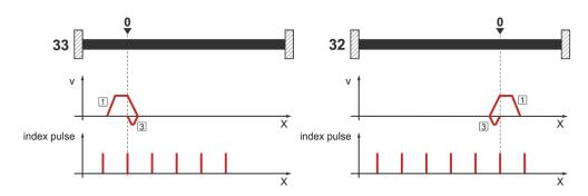
Figure 43: Index pulse with a negative (32) and positive (33) initial movement
