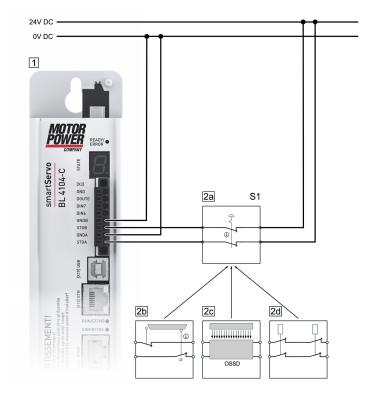
Figure 124: Connection of the integrated STO function (single-phase servo drive)
