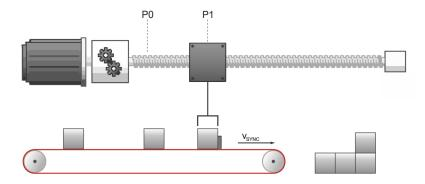
Figure 68: Gripping of the object and synchronous movement
