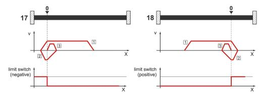
Figure 38: Homing run to the limit switch
