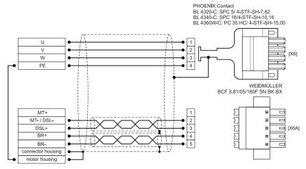
Figure 146: Pin assignment: motor connector (HIPERFACE DSL®) [X6], [X6A]
