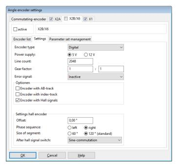
Figure 87: "Angle encoder settings" window - "X2B/X6" tab - "Settings" - "Encoder type: Digital"
