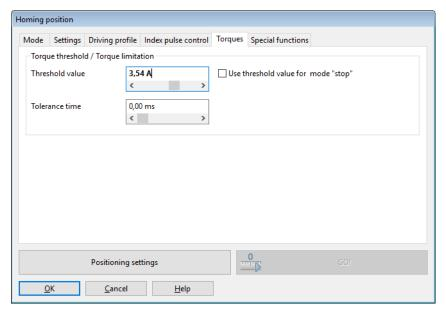
Figure 48: "Homing position" window - "Torques" tab
