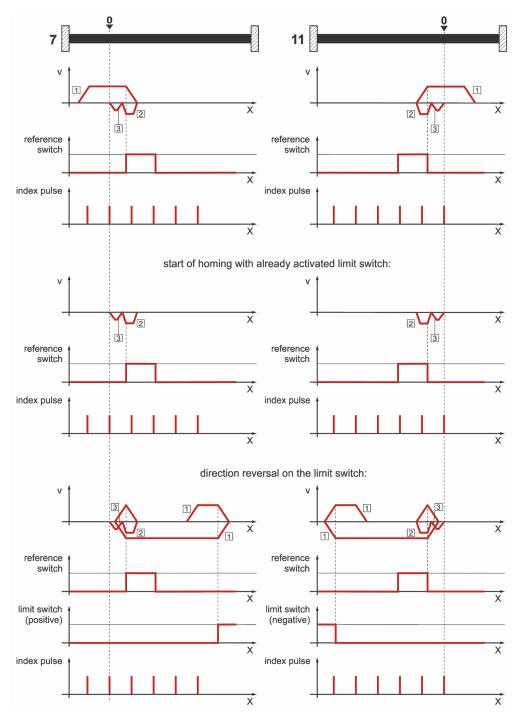
Figure 41: Homing run to the reference switch with index pulse evaluation
