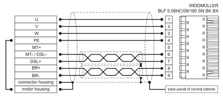
Figure 142: Pin assignment: motor connector (HIPERFACE DSL®) [X6]
