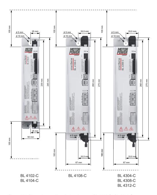
Figure 131: Dimensions and installation clearance BL 4102-C...BL 4312-C
