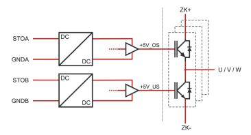
Figure 122: "Safe Torque Off" - principle of operation
