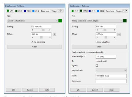
Figure 75: Oscilloscope" window - "CHx" tab
