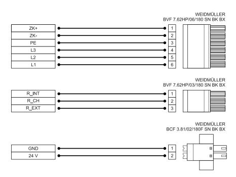
Figure 138: Pin assignment: "power supply connector [X9], [X9A], [X9B]"
