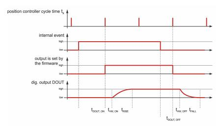
Figure 158: Filter time mechanism in the case of digital outputs
