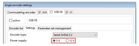
Figure 148: Angle encoder settings: Parameterisation of supply voltage
