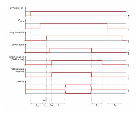
Figure 159: Time diagram of the servo drive
