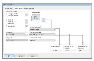
Figure 31: "Setpoint selectors" windows - "Speed control" tab
