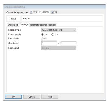
Figure 91: Angle encoder settings" window - "X2B/X6" tab - "Settings" - "Encoder type: Serial: HIPERFACE DSL"
