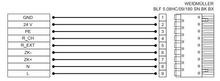
Figure 134: Pin assignment: "power supply connector [X9]"
