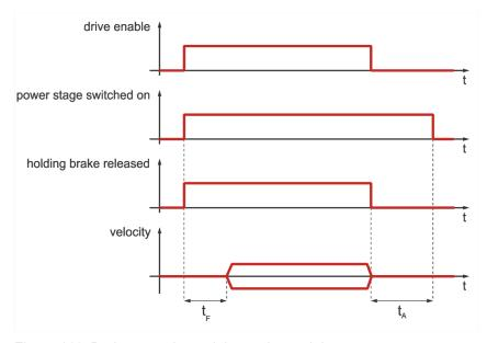
Figure 113: Brake control: run delay and stop delay
