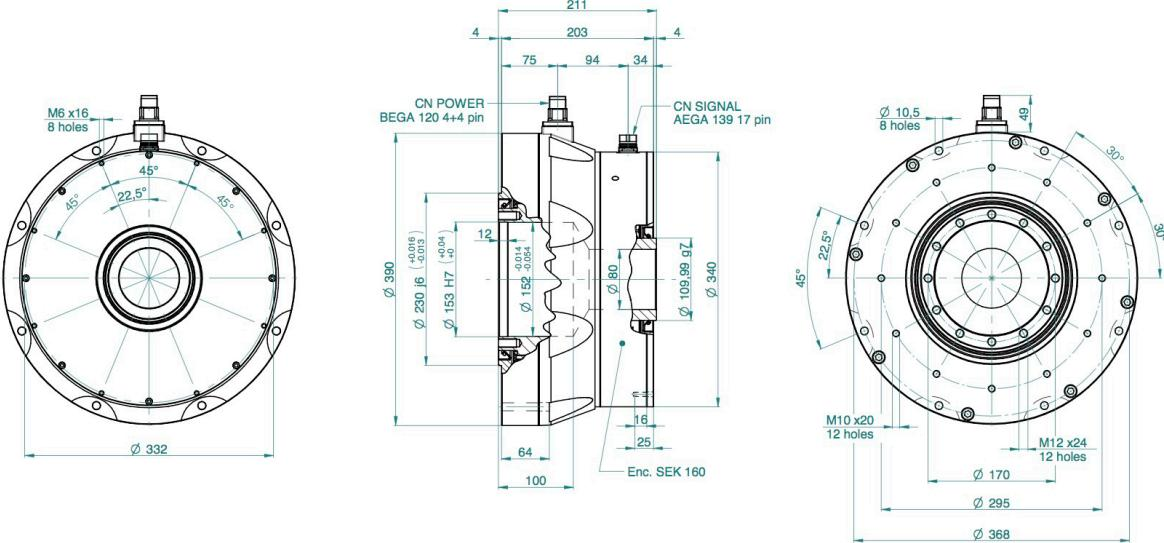
**SKA DDR 335 90 POWER PACK HOLLOW SHAFT reference drawing 305**
