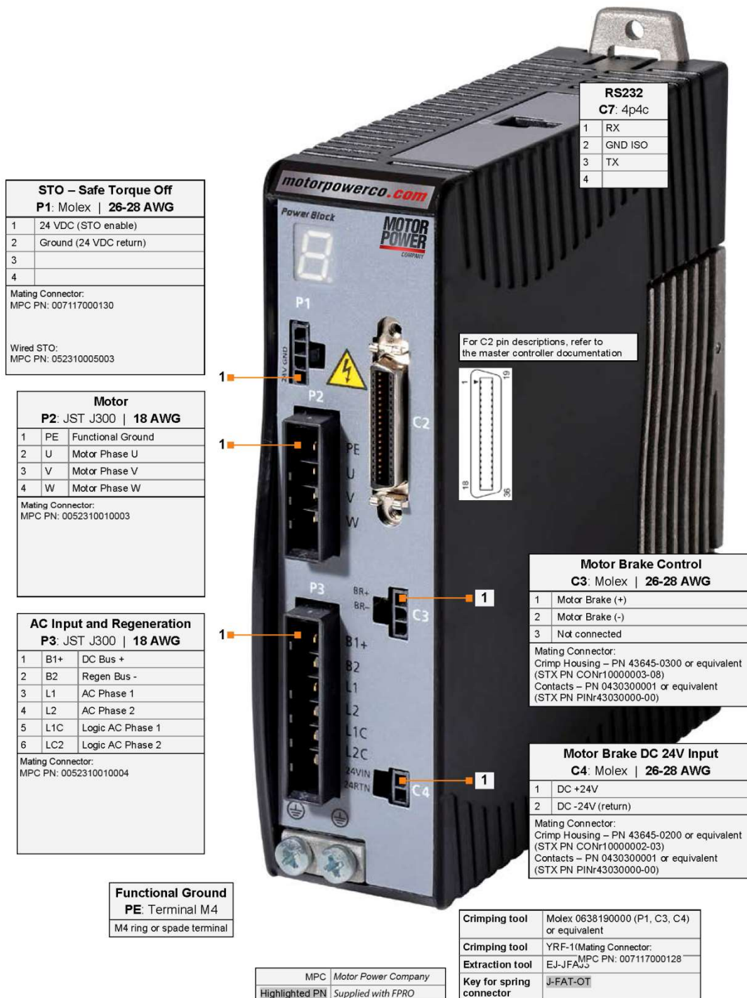
Figure 4-4. Pin Assignments on FLEXI PRO-1D5/FLEXI PRO-003 – PB Models (120/240 VAC)
